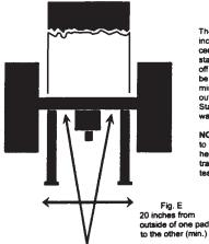
The stabilizer bar will extend a minimum of 32 inches behind a line (Fig. A) drawn from the center of the wheel (Fig. B) to the ground. The stabilizer pad must be no more than 10 inches off the ground (Fig. C). The stabilizer pad must be a minimum of five inches square (Fig. D). A minimum of 20 inches will be allowed from the outside of one pad to the other (Fig. E). Stabilizer bars are not to be mounted in any way to the drawbar.
